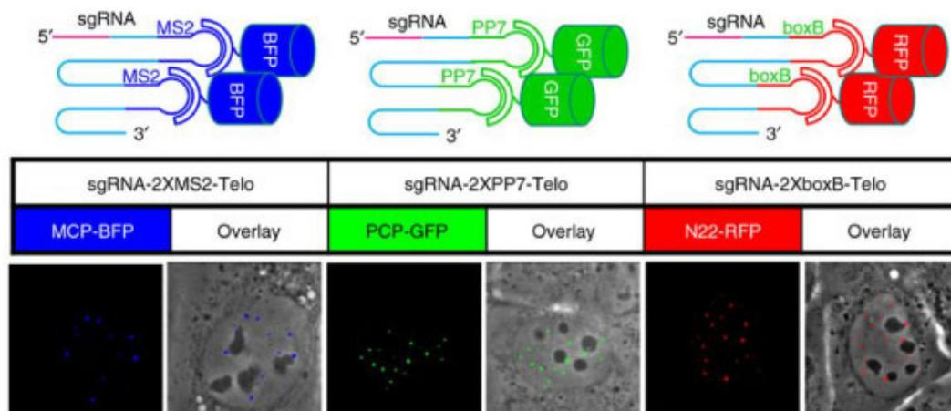
Figure 1: CRISPRainbow labeling. Two MS2, PP7, or boxB sequences inserted into the sgRNA generates blue, green, or red colors for labeling. A combination of MS2, PP7, or boxB sequences in the same sgRNA will generate additional colors. Image from [Ma et al., 2016](#) with permission.
